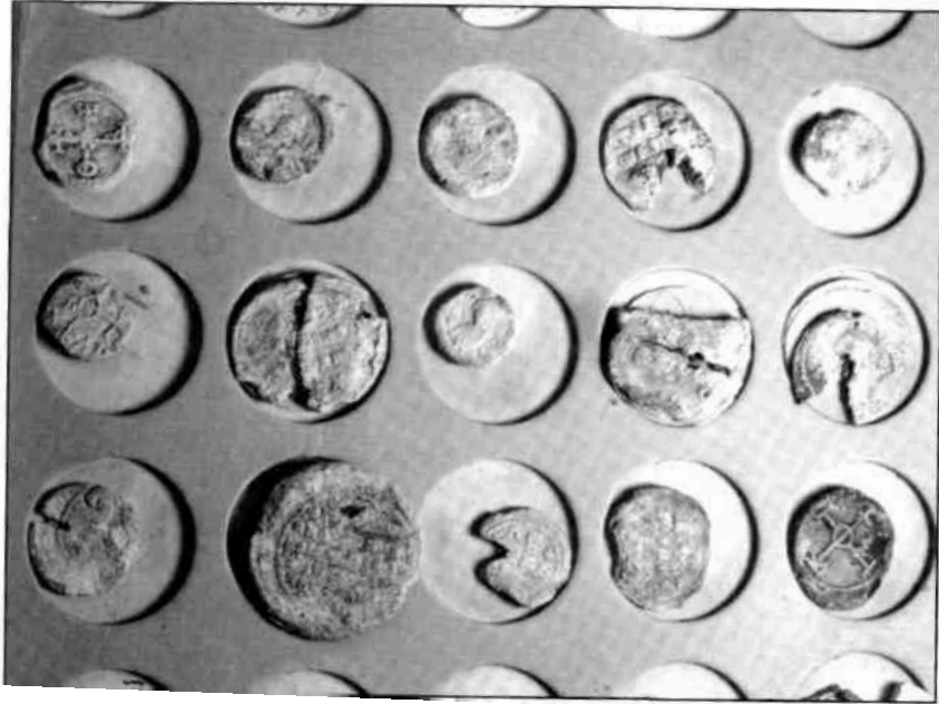
FIG. 1. An old cardboard tray with lead seals of the Museum's, collections. The adverse storage conditions caused disintegration of their surface.
